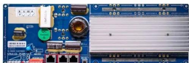
RS485 * Communication between battery and inverter Read rate: 1000bps RS485 Interface * Communication between parallel packs or BMS and PC Read rate: 5000bps
